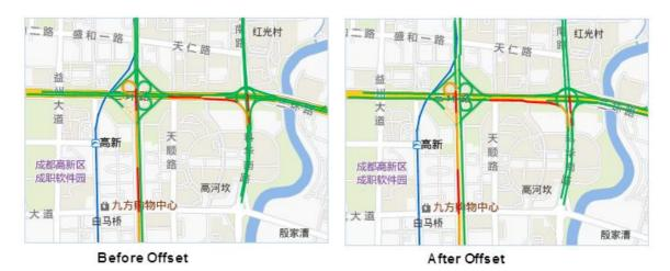
When zooming out the scale, the roads may be overlapped, and the congestion condition can't be seen clearly. If users want to display the condition of the double-way roads clearly at small scale, SuperMap provides the Traffic Line Correction function to improve the display effect, which will determine whether to display the traffic condition and process the offset values, please refer to Traffic Line Correction.
